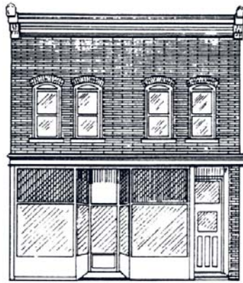
Example of Commercial Vernacular Style
